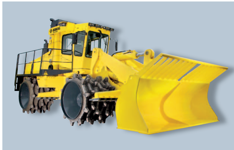
RS version with lifting gear and bucket.
