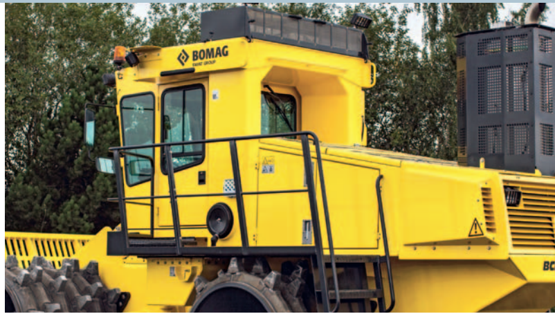
The service platform gives access to the maintenance area.
