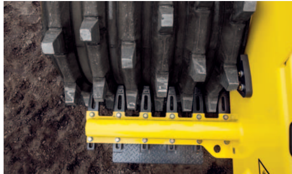
Adjustable scraper for uninterrupted operations.
