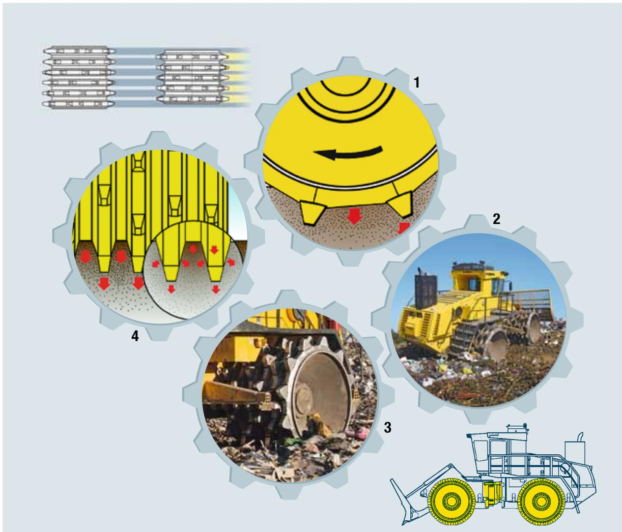
**1** Polygonal disc wheels with teeth for maximum crushing, kneading, depth effect and compaction.
