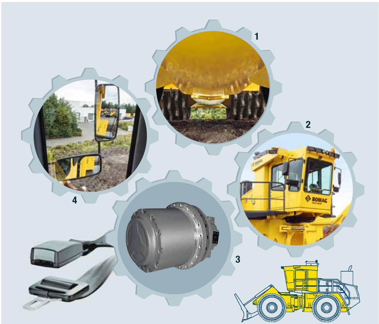
**1** Frame in enclosed box design offers maximum protection to all drive units with no material ingress, i.e. no ignition on hot components.
