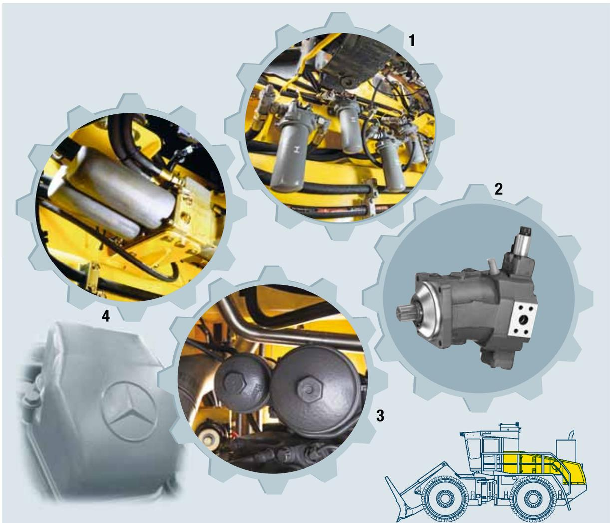
**1** Filter system in the hydraulics.
