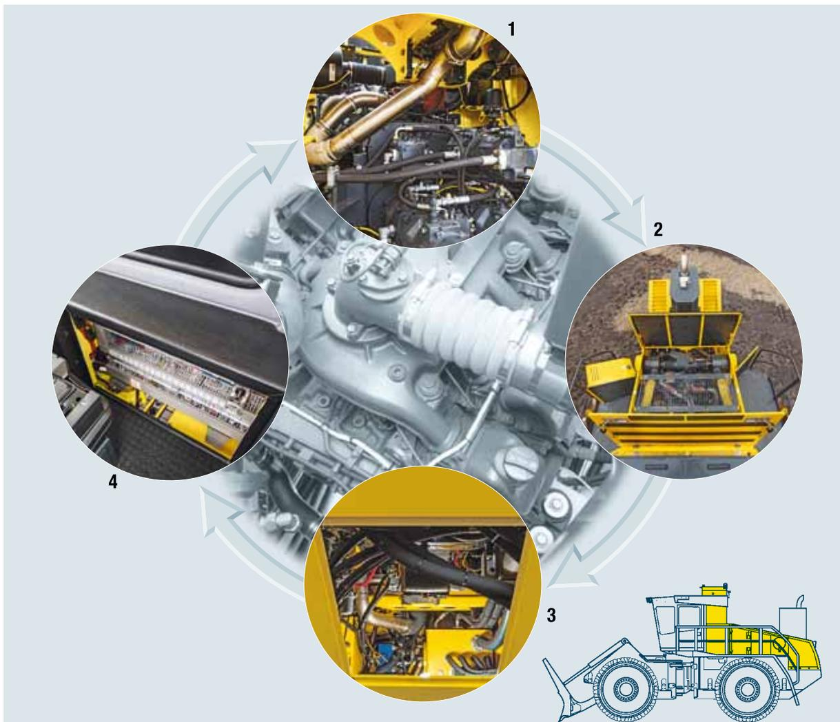
**1 Large maintenance openings** for easy access to the drive components.
