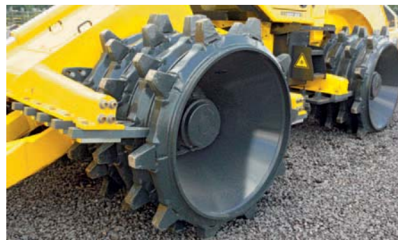
Welded wheel sections with inner taper on both sides for optimum stability.
