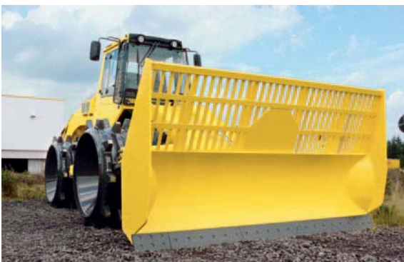
Refuse compactor with dozer blade...
