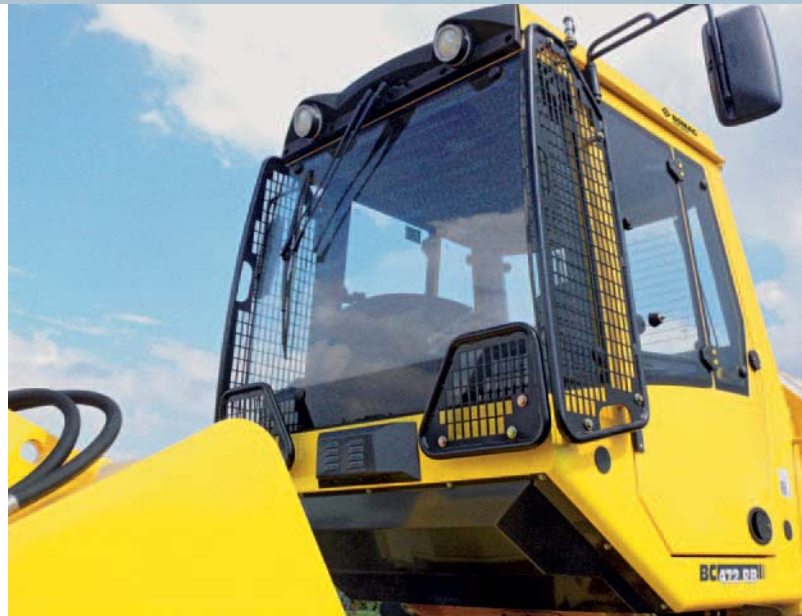
A front grid protects the screen from damage.
