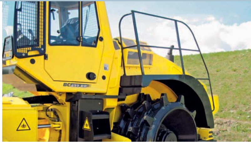
The service platform provides access to the maintenance area.
